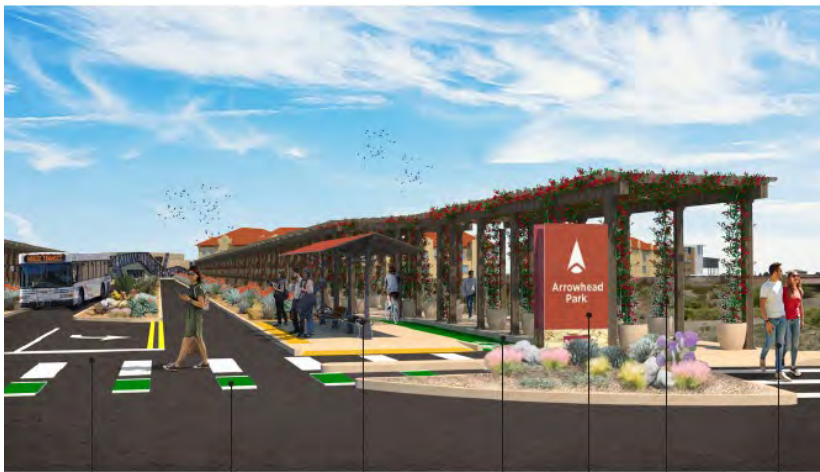
Turning lane Cross Markings to raise awareness Transit stop Protected Bike Lane Signage Shaded Sidewalk Trellis Access to Arroyo Trail
